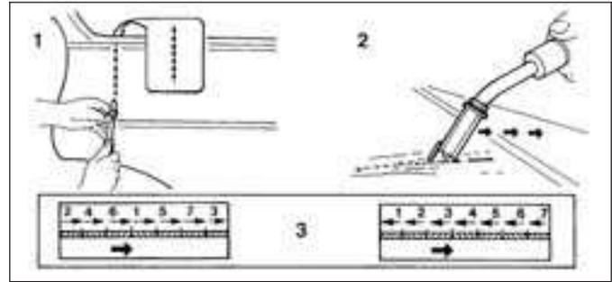
The difficulty in carrying out a single seam weld is that the torch must be moved fairly slowly to produce good penetration of the weld but sufficiently quickly so as not to run the risk of "burning" the panel.
