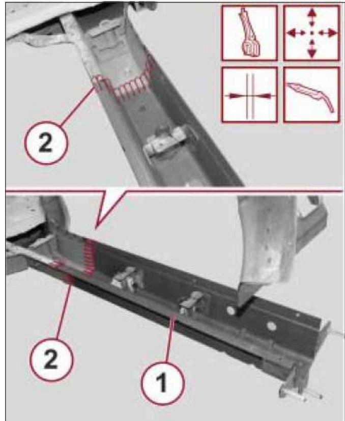
7. Correct any distortions to the sheet metal using a hammer and dolly block.
