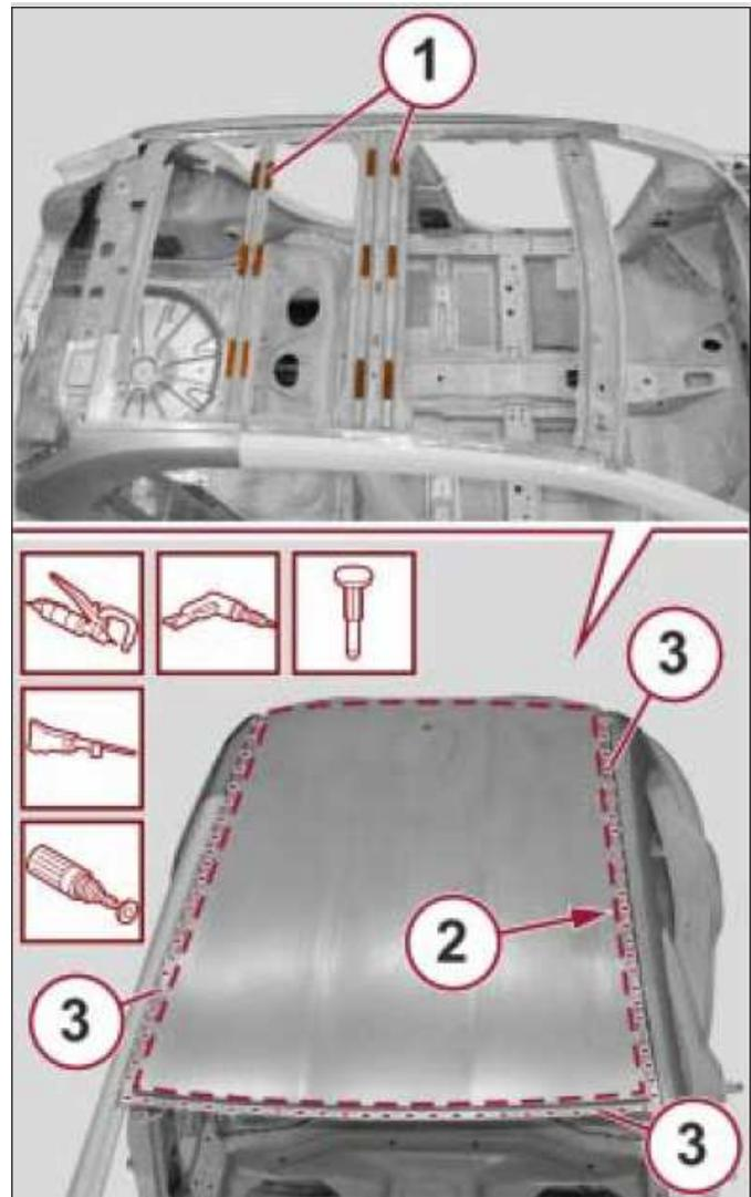
10. With the use of a reciprocating saw, cut the roof along the cut line (1) using care not headers and roof bows.
