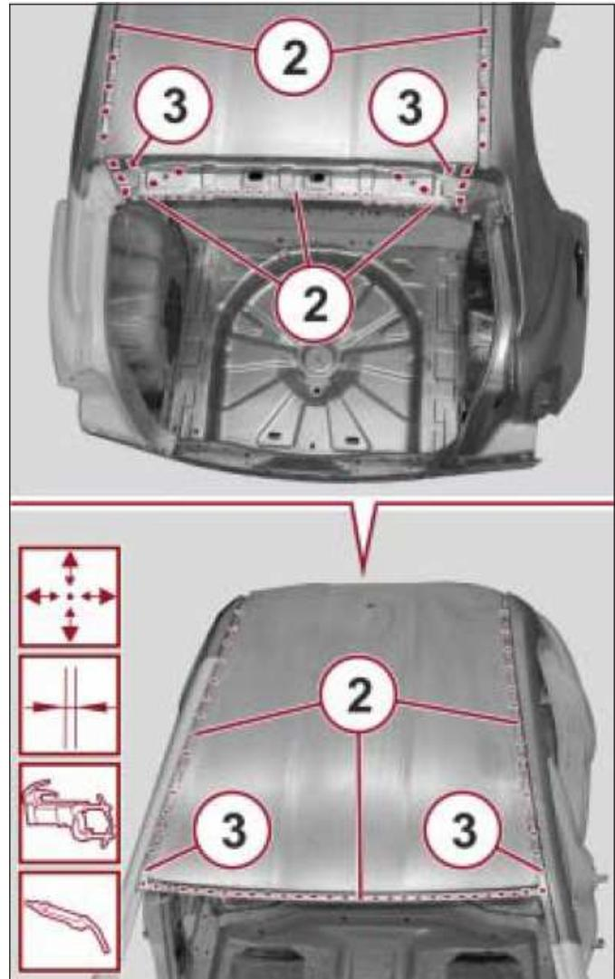
9. Correct any distortions of the panel using a hammer and dolly block.
