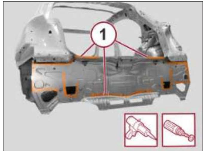
13. With the use of a rotary brush, remove the anti-corrosion treatment around the entire perimeter (1) of the inside and outside of the outer service part (1).
