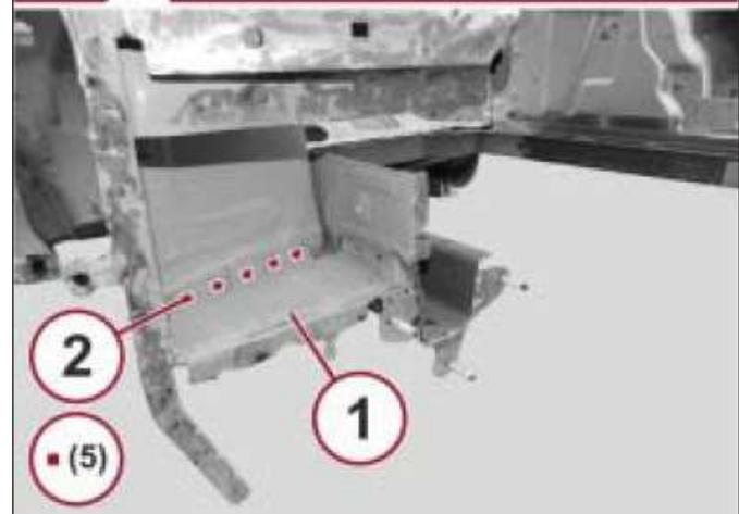
8. Use a disc grinder to smooth the welds.
