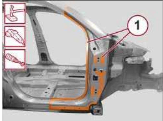
38. Apply corrosion protection to the areas involved in the welding.
