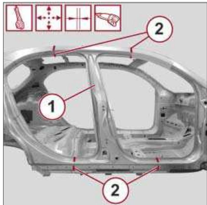
36. Position the b-pillar external service part correctly on the vehicle and secure it with the self-locking clamps.
