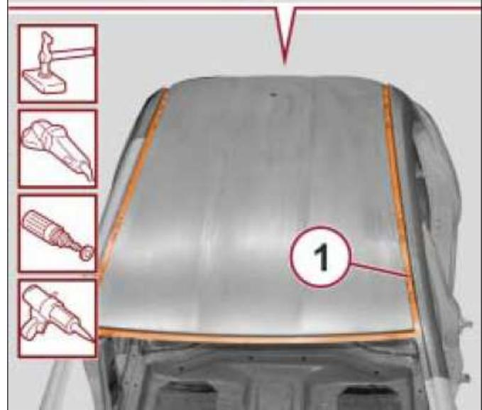
4. With the use of a rotary brush, remove the paint and access to the spot welds.
