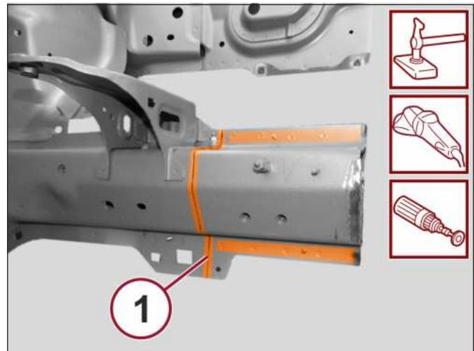
15. Correct any distortions to the sheet metal using a hammer and dolly block.
