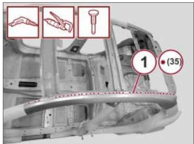
14. With the use of a hammer and dolly block, straighten the edges of the mating components.
