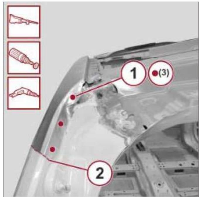
10. With the use of a spot weld cutting tool, release the spot welds (1).
