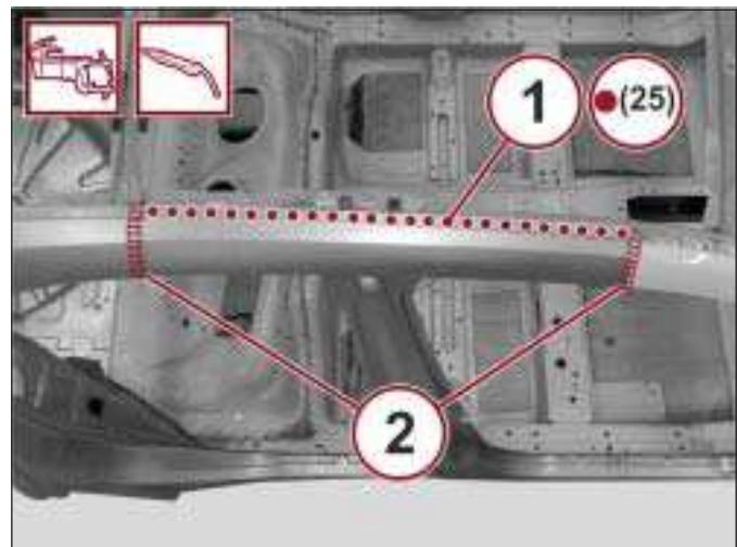
43. Correct any distortions to the sheet metal using a hammer and dolly block.
