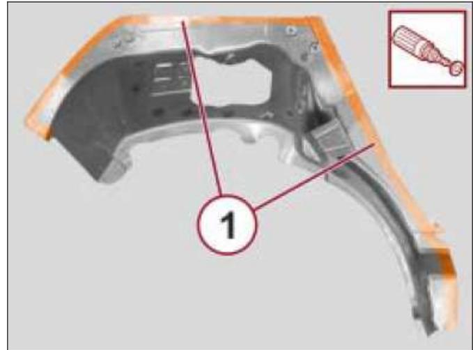
2. With the use of a drill, drill holes at the indicated points (1).
