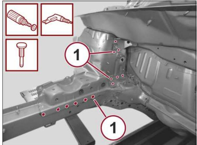
8. Use a rotary brush to remove the paint and gain access to the spot welds (1).
