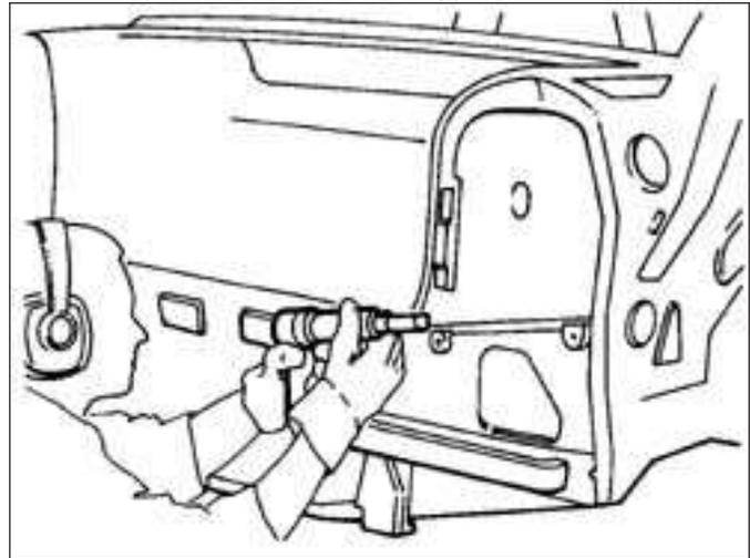
**Example of application of pneumatic chisel.**
