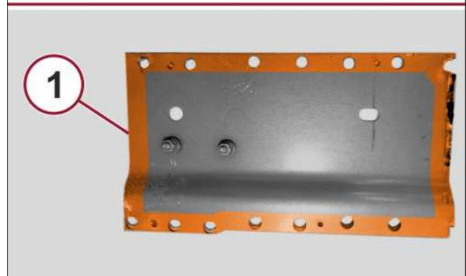
5. Create and install 50 mm (2 in.) backer panels to the butt joint areas (2).
