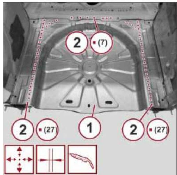
8. With the use of a disc grinder, smooth the welds in the affected area (1).
