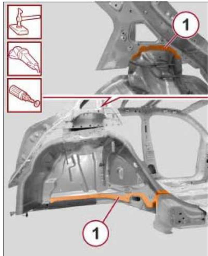
12. Apply corrosion protection to the areas (1) involved in the welding.
