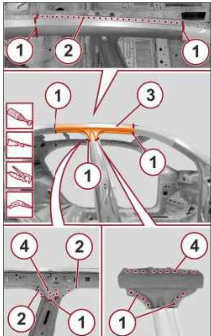
10. With the use of a rotary brush, remove the paint and gain access to the spot welds.
