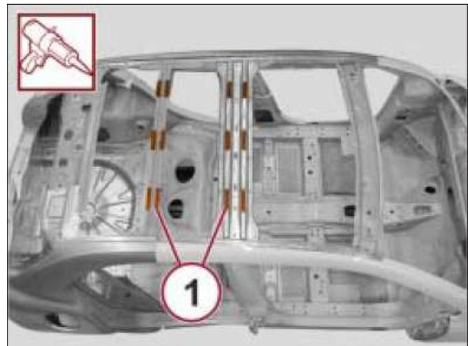
5. Position the service part correctly on the vehicle and secure it with the self-locking clamps.
