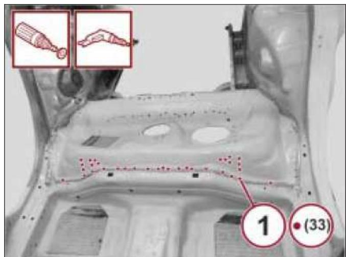
11. Use a chisel and hammer to remove the previously released spot welds.
