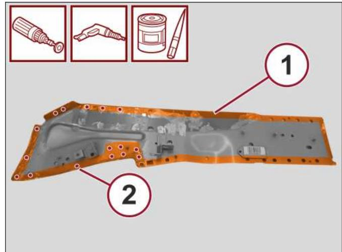
7. Remove the anti-corrosion treatment from the entire perimeter of the inside and outside of the service part internal (1) using a rotary brush.
