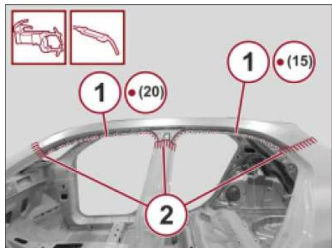
18. Correct any distortions to the sheet metal using a hammer and dolly block.
