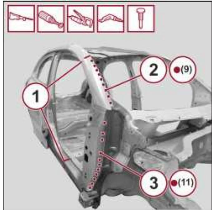
16. With the use of a rotary brush, remove the paint and gain access to the spot welds.
