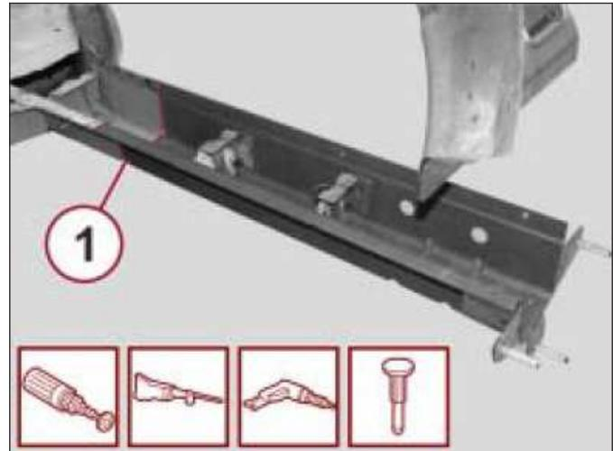
18. With the use of a hammer and dolly block, straighten the edges of the mating components.
