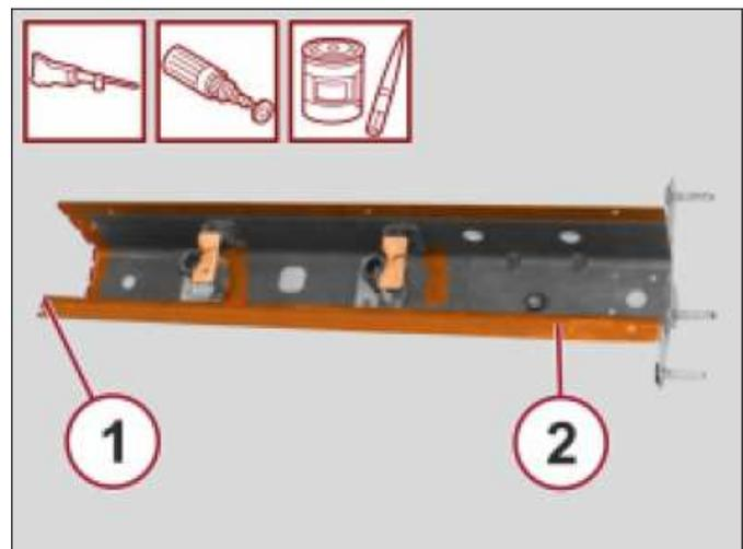
4. Position the service part (1) correctly on the vehicle and secure it with the self-locking clamps.
