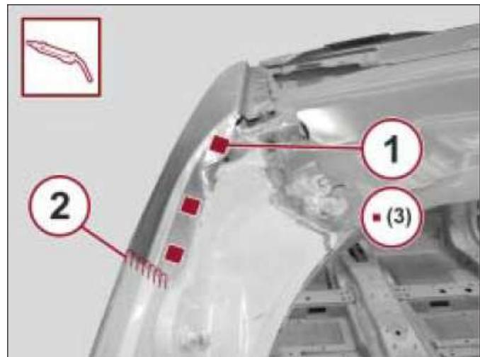
16. With the use of a spot welder, apply spot welds to the areas (1) indicated in the figure.
