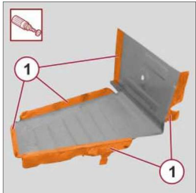
2. With the service part placed on a workbench, use a drill to drill holes (1) in the area shown.
