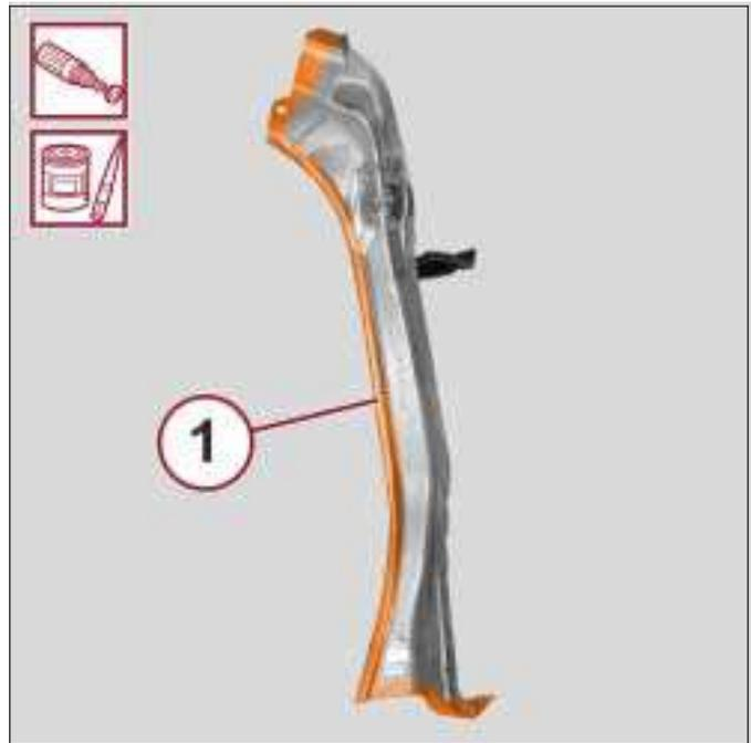
3. Position the service part correctly on the vehicle and secure it with the self-locking clamps.
