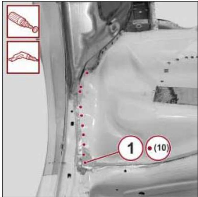
9. With the use of a drill, remove the spot welds (1) shown in the figure.
