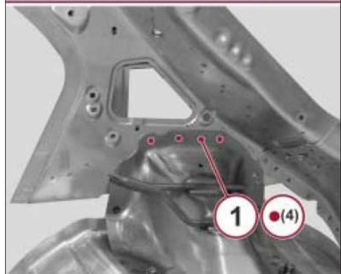
17. With the use of a hammer and dolly block, straighten the edges of the mating components.
