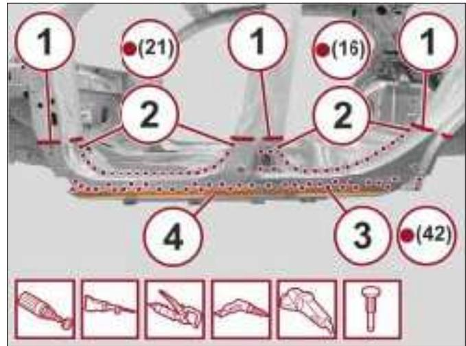
11. With the use of a drill, release the spot welds (1) shown in the figure.
