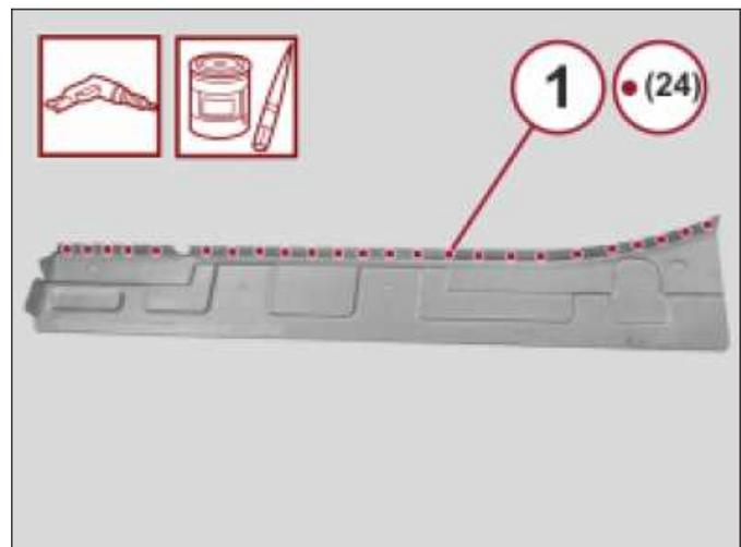
4. Position the service part (1) correctly on the rear frame rail and floor pan.
