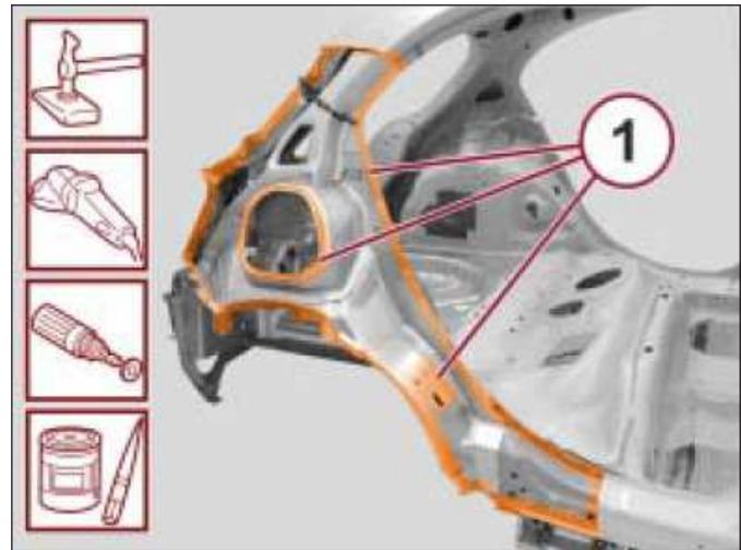
16. With the use of a hammer and dolly block, straighten the edges (1) of the mating components.
