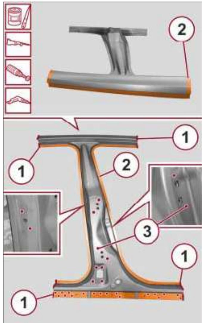
31. Position the service part correctly on the vehicle and secure it with the self-locking clamps.
