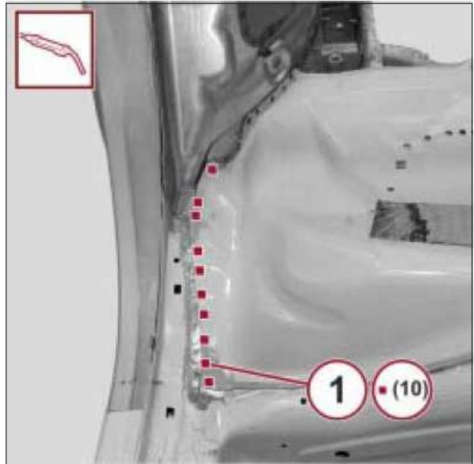
9. With the use of a MIG welder, apply plug welds to the areas (1) shown in the figure.
