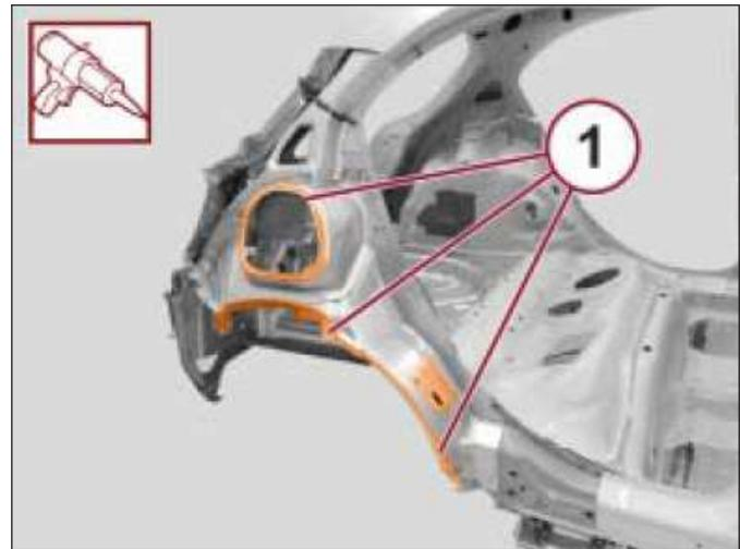
11. Position the service part correctly on the vehicle and secure it with the self-locking clamps.
