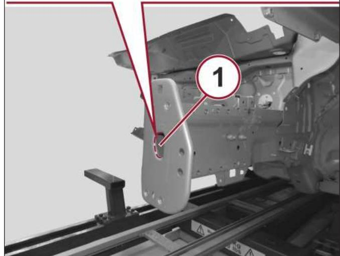
6. Straighten the edges of the front frame rail with the use of a hammer and dolly block.
