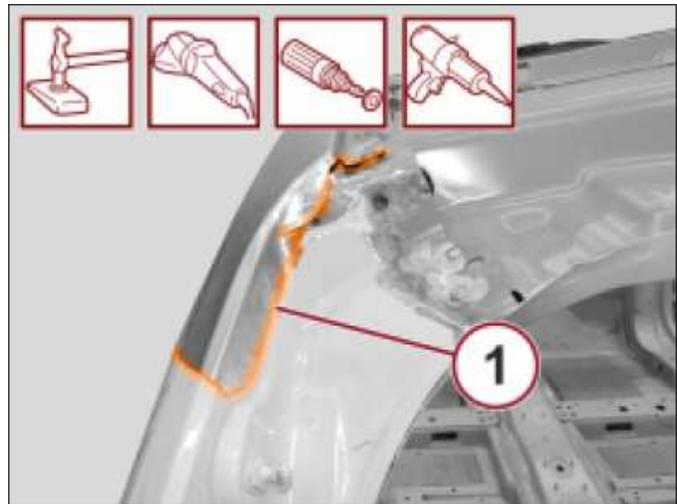
28. Correct any distortions to the sheet metal using a hammer and dolly block.
