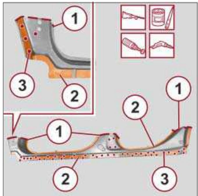
5. Position the outer service part (1) correctly on the vehicle and secure it with the self-locking clamps.
