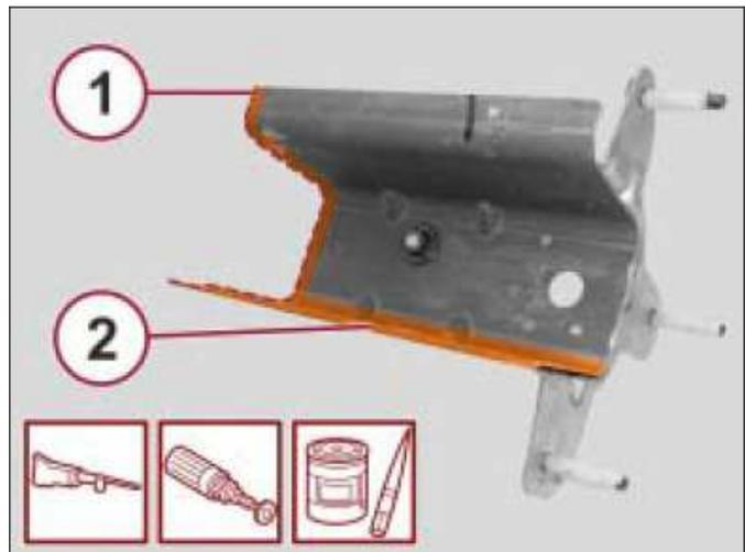
4. Position the service part correctly on the vehicle and secure it with the self-locking clamps.
