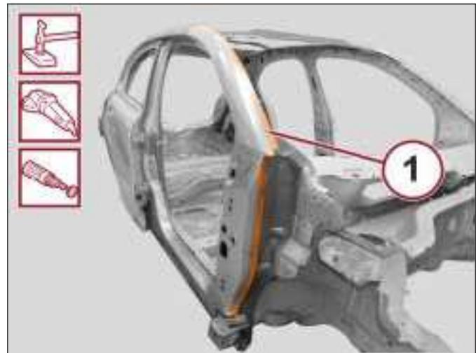
35. Correct any distortions to the sheet metal using a hammer and dolly block.
