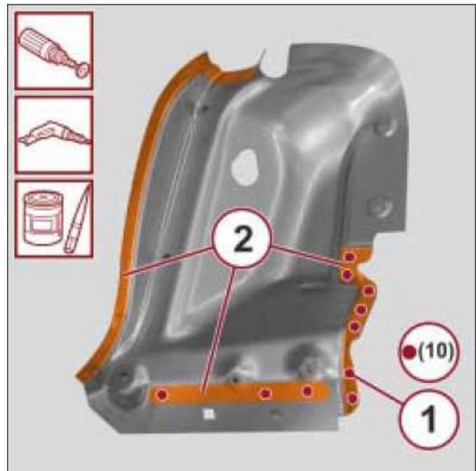
4. Position the service part correctly on the vehicle and secure it with the self-locking clamps.
