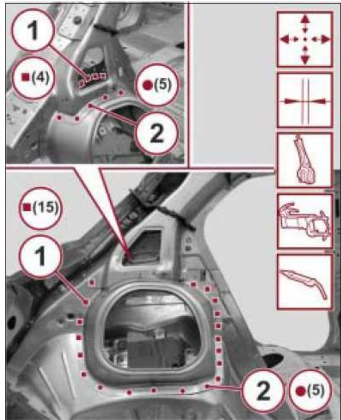
9. Correct any distortions to the sheet metal using a hammer and dolly block.
