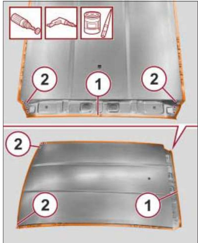
4. Apply a beads of sealant (1) along the roof bows.
