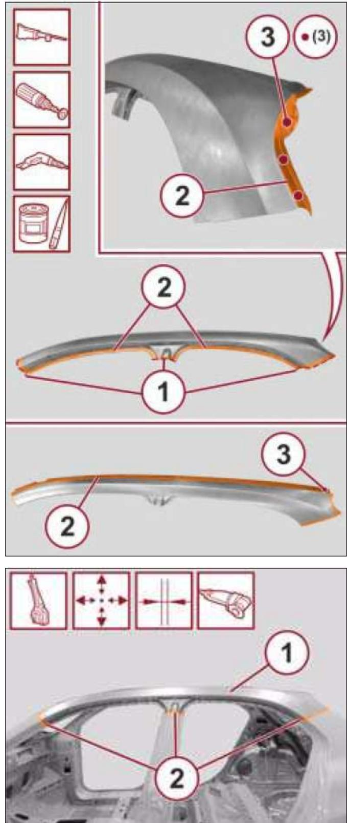
5. Position the service part (1) correctly on the vehicle and secure it with the self-locking clamps.
