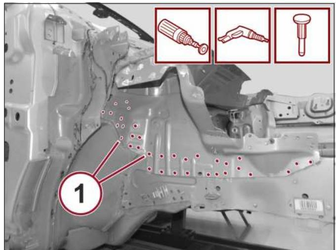
11. Use a rotary brush to remove the paint and gain access to the spot welds (1).
