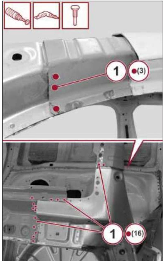
14. With the use of a rotary brush, remove the paint and gain access to the spot welds.
