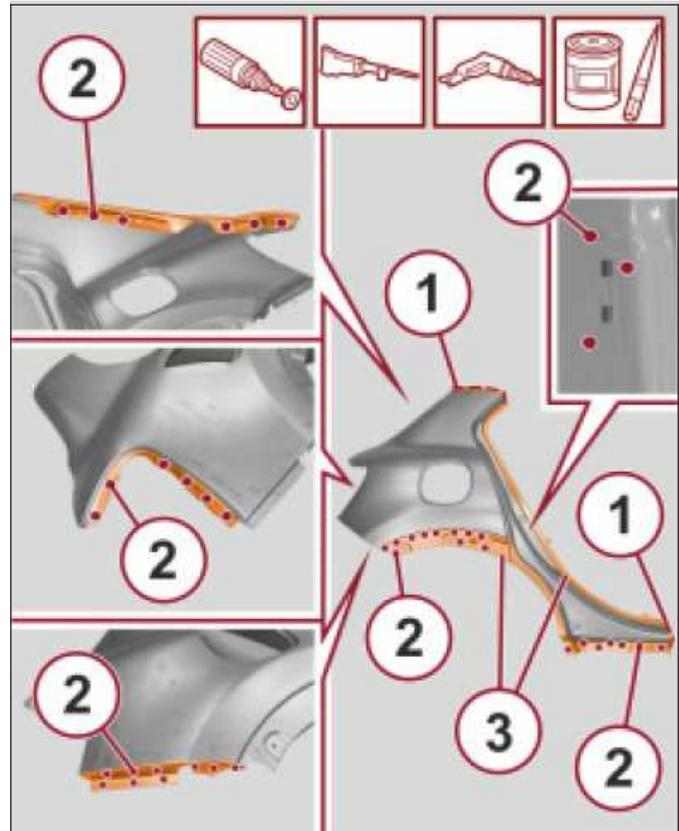
5. Position the service part (1) correctly on the vehicle and secure it with the self locking clamps.
