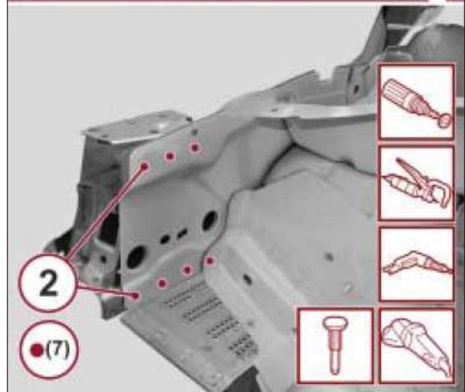
11. With the use of a drill, release the spot welds (1) shown in the figure.
