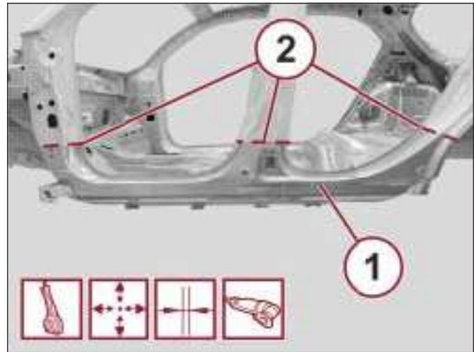
10. Position the body side aperture sill service part correctly on the vehicle and secure it with the self-locking clamps.
