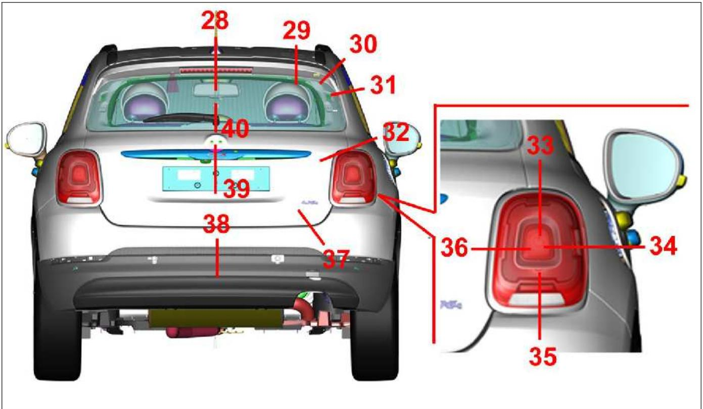
Rear view of the vehicle with the position for measuring the gaps between the moving parts
