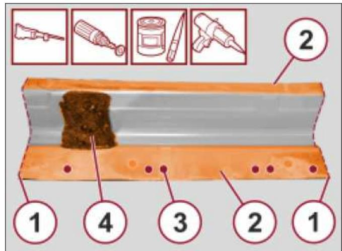
6. Position the service part (1) correctly on the vehicle and secure it with the self-locking clamps.
