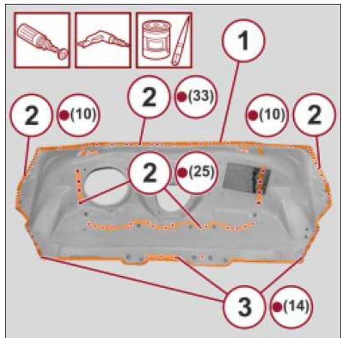
5. Position the center floor pan service part correctly on the vehicle and secure it with the self-locking clamps.
