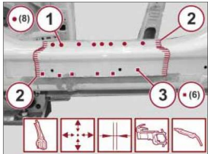
16. Correct any distortions to the sheet metal using a hammer and dolly block.
