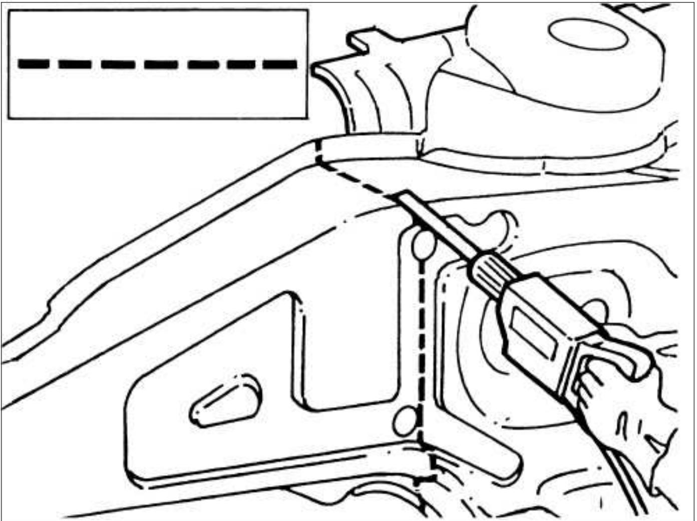
Cutting with a power saw or chisel
