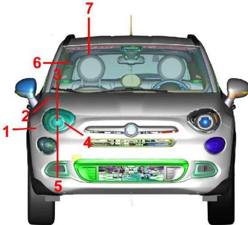
Front view of the vehicle with the position for measuring the gaps between the moving parts
