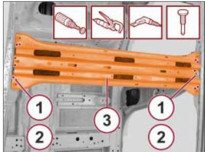
9. With the use of a disc grinder, remove any residue of the spot welds.
