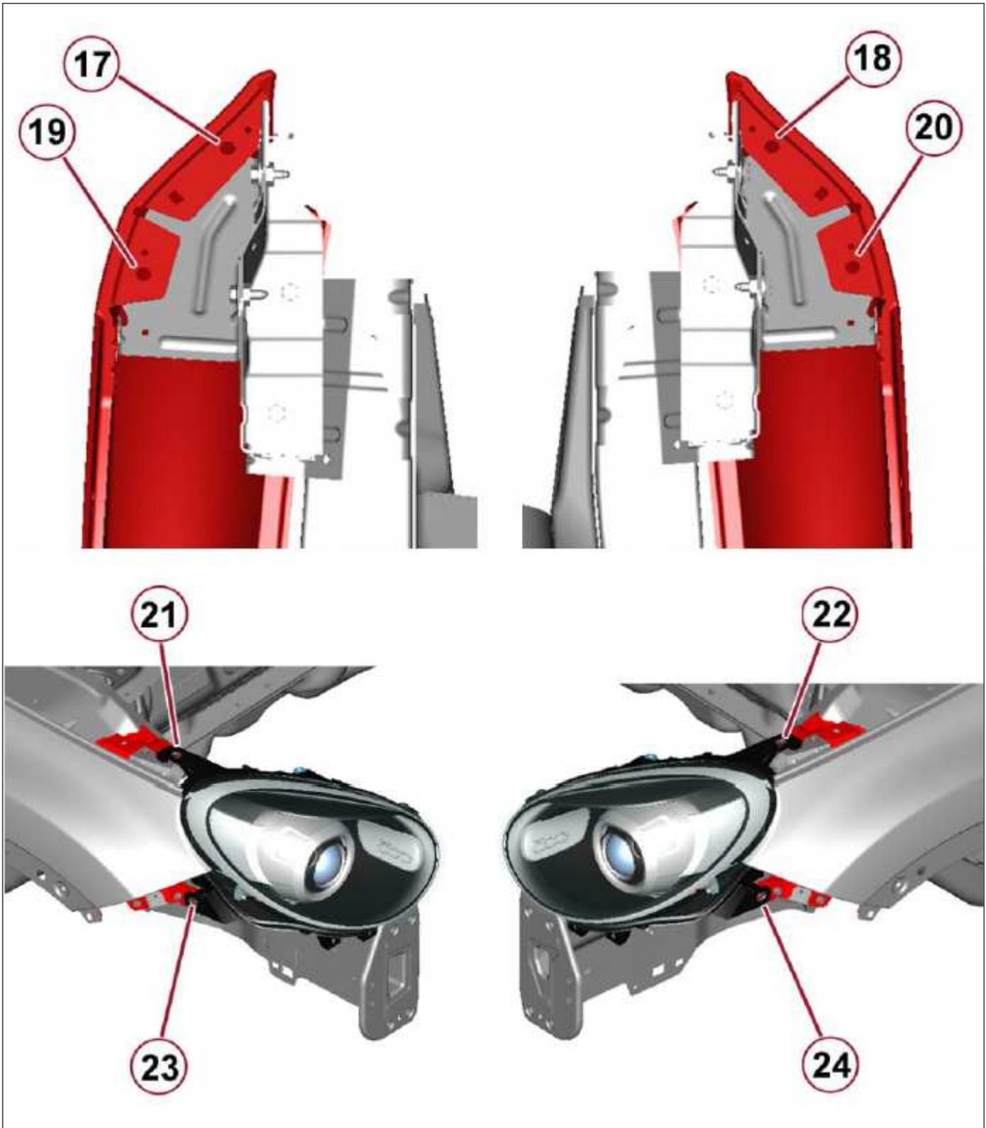
Fascia mounting to fender and headlight to body– View 1 of 2
