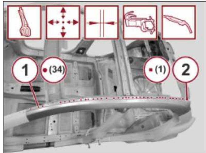
14. With the use of a MIG welder, apply plug welds filling in the areas (1) shown in the figure.
