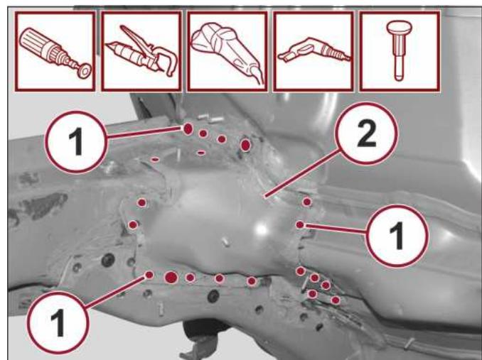
15. Use a rotary brush to remove the paint and gain access to the spot welds.
