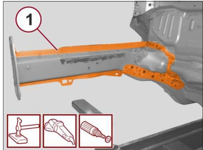
23. Correct any distortions to the panel using a hammer and dolly block.
