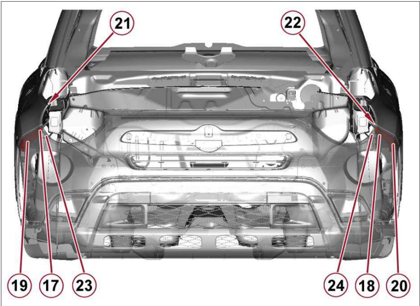
Fascia mounting to fender and headlight to body– View 2 of 2
