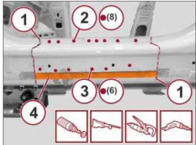
8. With the use of a hammer and dolly block, straighten the edges of the mating components.
