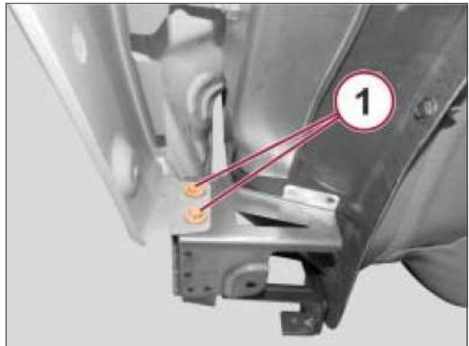
11. Remove the two lower bolts (1) securing the fender (2) to the support bracket.
