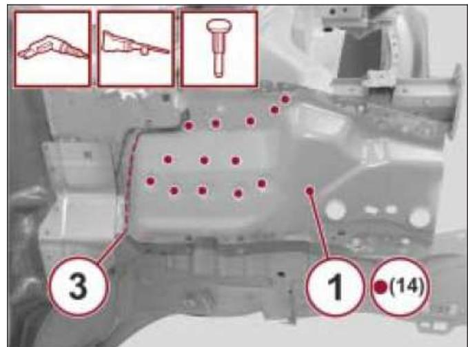
15. With the use of a hammer and dolly block, straighten the edges (1) of the mating components.
