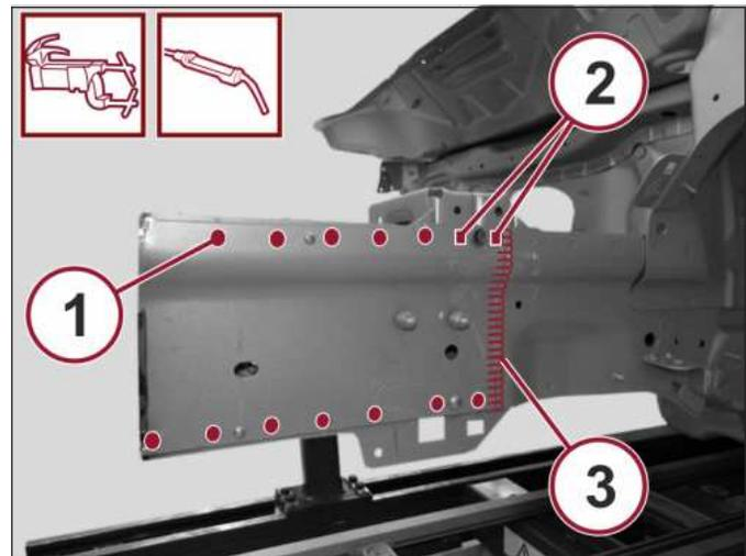
12. Correct any distortions to the sheet metal using a hammer and dolly block.
