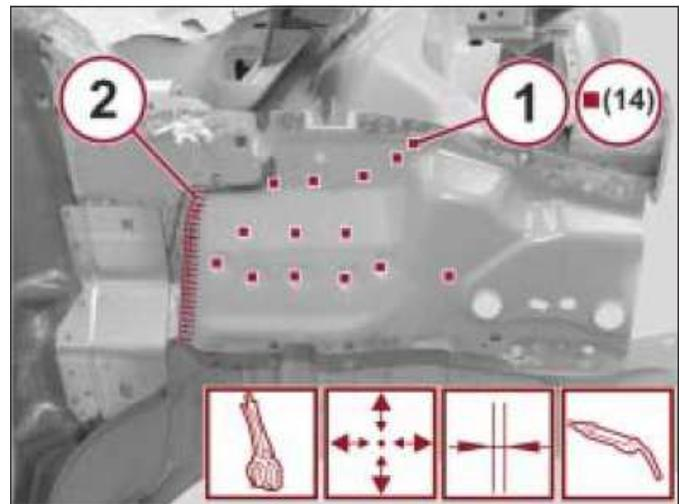
12. Position the outer service part correctly on the vehicle and secure it with the self-locking clamps.
