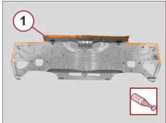
2. Drill out the internal service part at the points (1) indicated.
