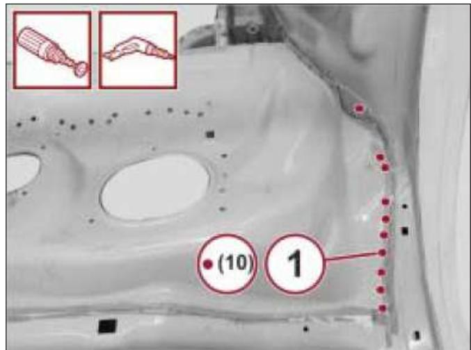
10. With the use of a drill, remove the spot welds (1) shown in the figure.
