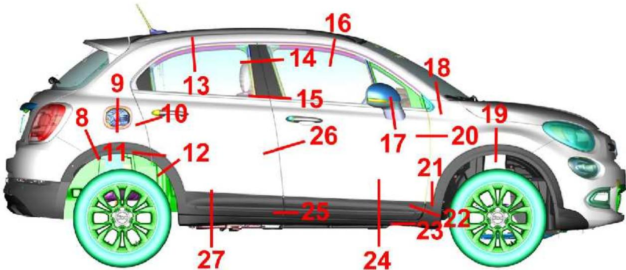
Side view of the vehicle with the position for measuring the gaps between the moving parts
