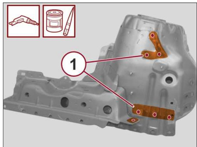
8. Position the service parts (1) correctly on the vehicle and secure it with the self-locking clamps.
