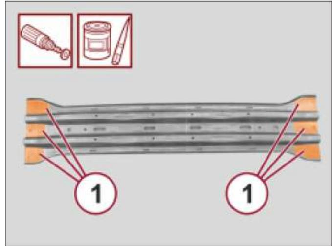
3. Position the service part (1) correctly on the vehicle and secure it with the self-locking clamps.
