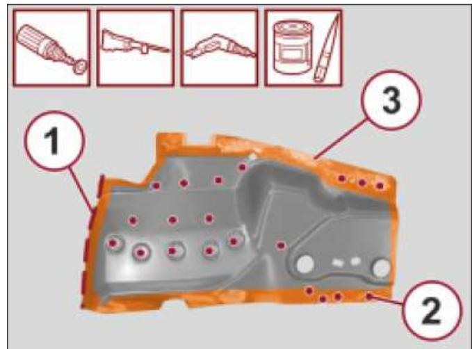
5. With the use of a rotary brush, remove the anti-corrosion treatment around the entire perimeter of the inside and outside of the outer service part.
