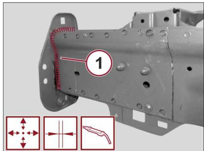
5. Correct any distortions to the sheet metal using a hammer and dolly block.
