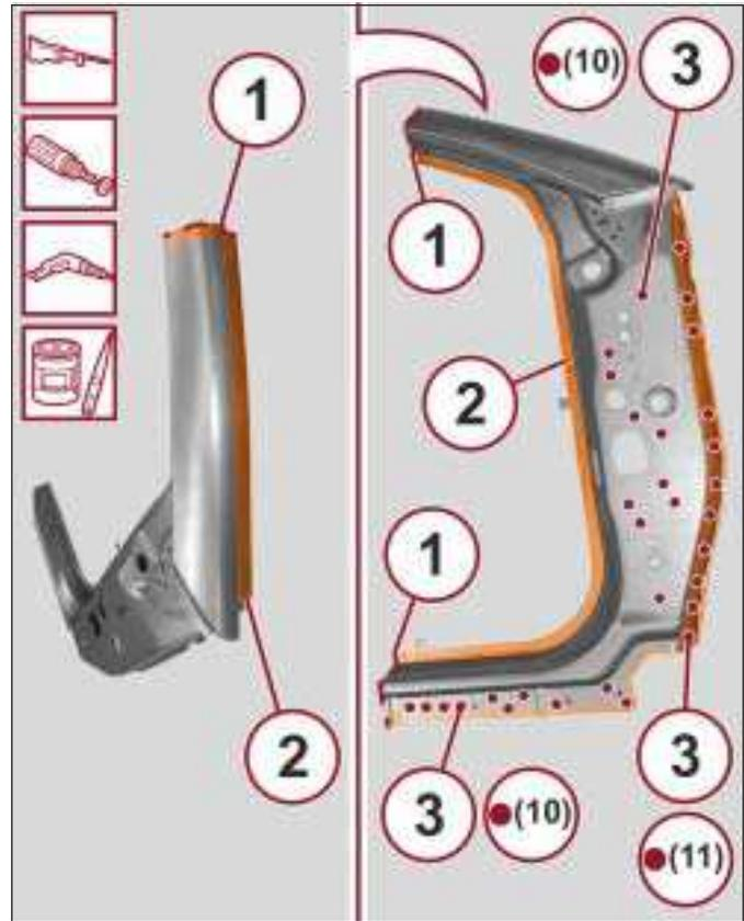
8. Position the cowl side reinforcement correctly on the vehicle and secure it with the self-locking clamps.
