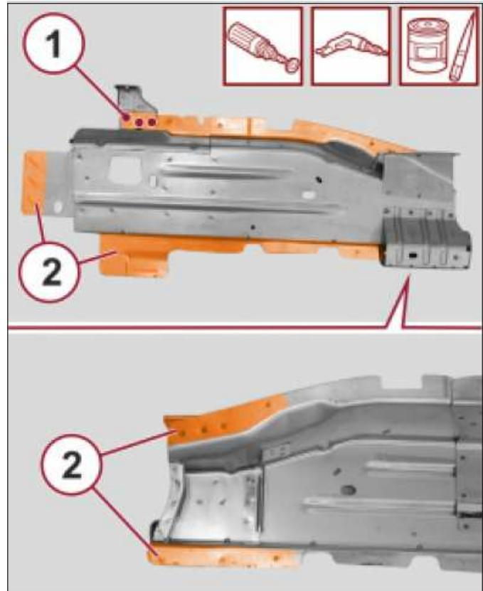
8. Position the inner service part correctly on the vehicle and secure it with the self-locking clamps.
