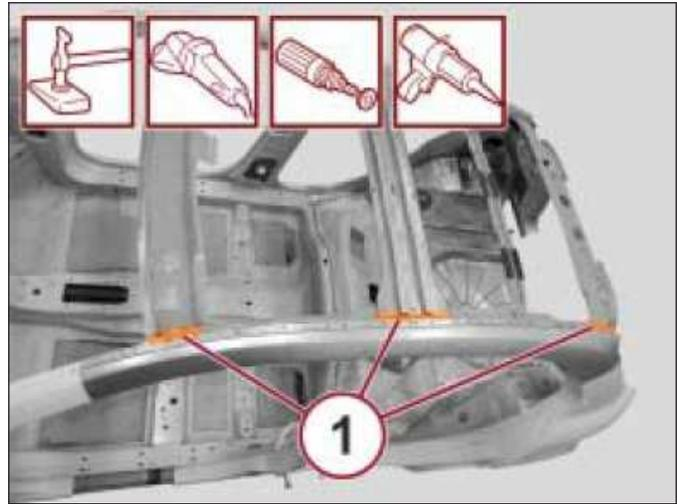
23. Correct any distortions to the sheet metal using a hammer and dolly block.
