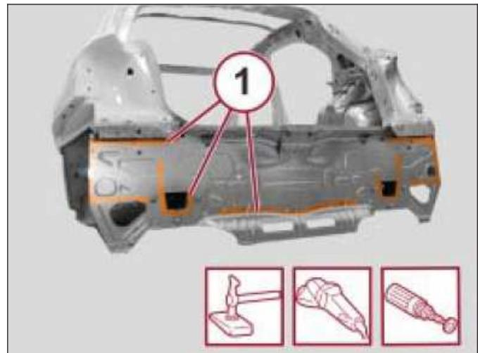
11. Apply corrosion protection to the areas (1) involved in the welding.
