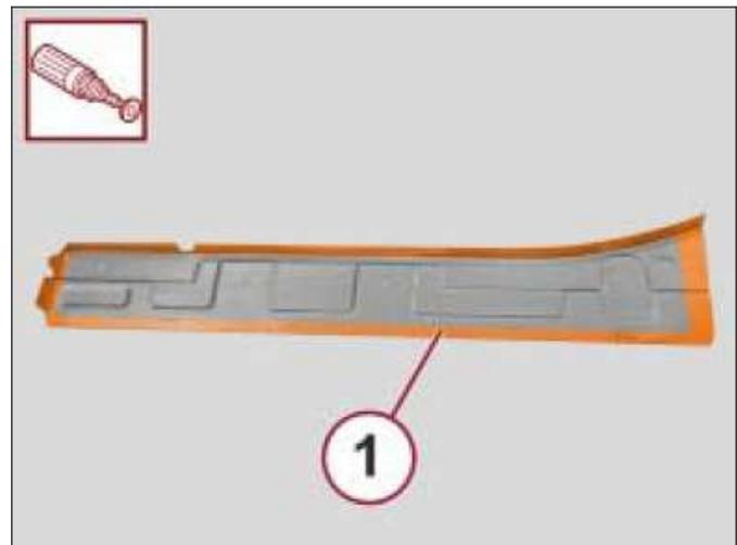
2. With the use of a drill and the service part placed on a work bench, drill holes at the points (1) indicated.
