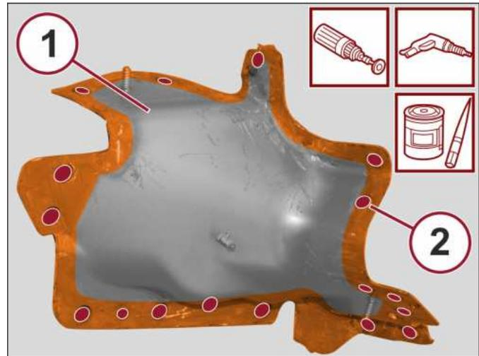
4. Remove the anti-corrosion treatment from the entire perimeter (1) of the inside and outside part using a rotary brush.
