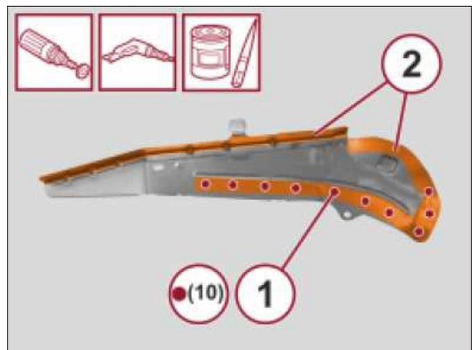
4. Position the part correctly on the vehicle and secure it with the self-locking clamps.
