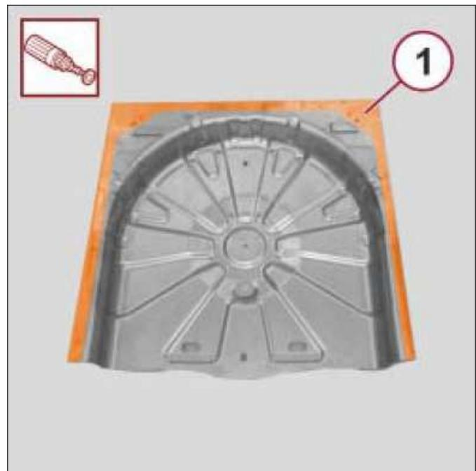
2. With the service part positioned on a work bench, drill the service part in line to the spot welds (1).
