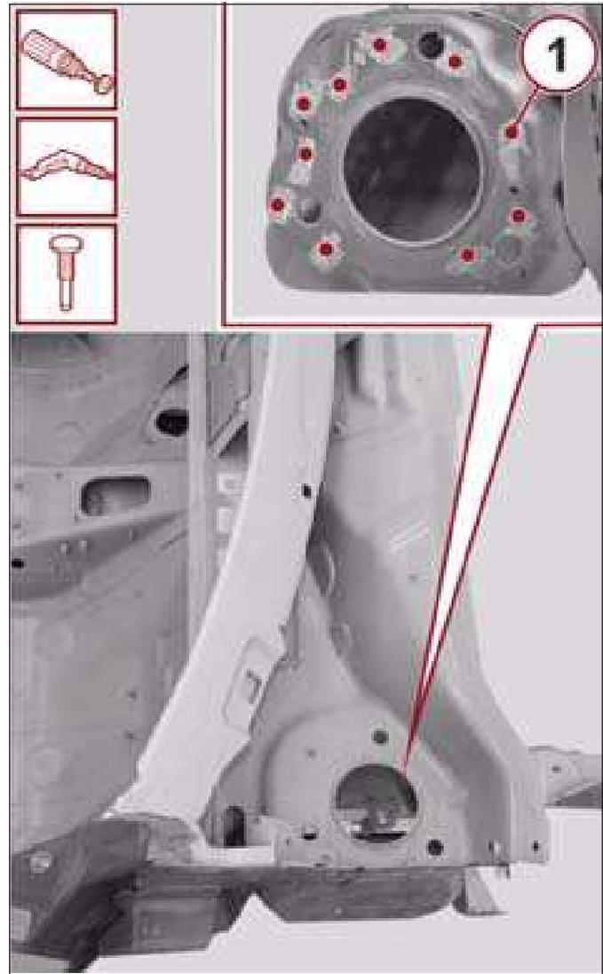
15. With the use of a hammer and dolly, straighten the edges of the mating components.
