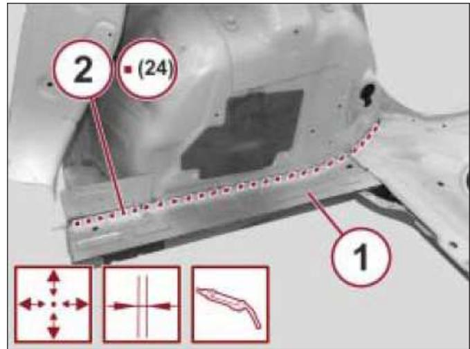
7. With the use of a disc grinder, smooth the welds.
