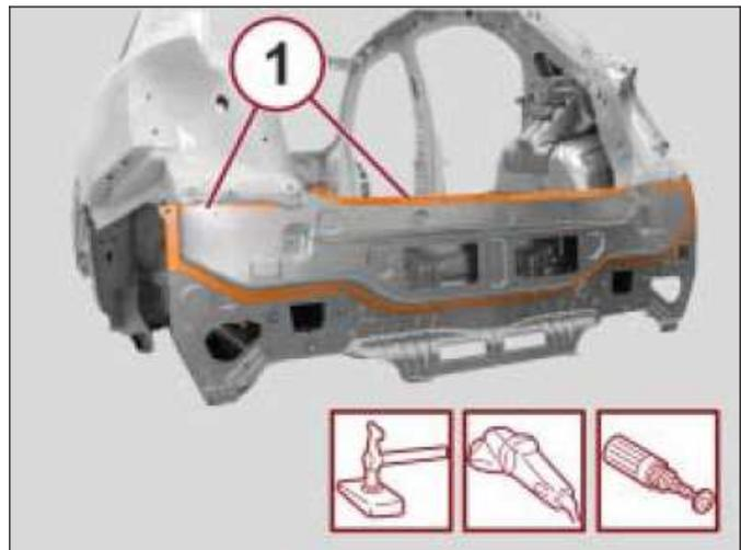
21. Apply corrosion protection to the areas (1) involved in the welding.
