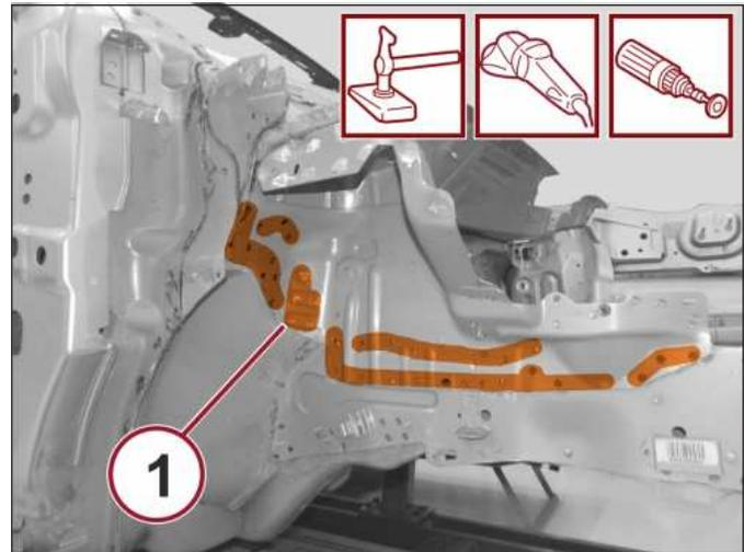
21. Correct any distortions to the panel using a hammer and dolly block.
