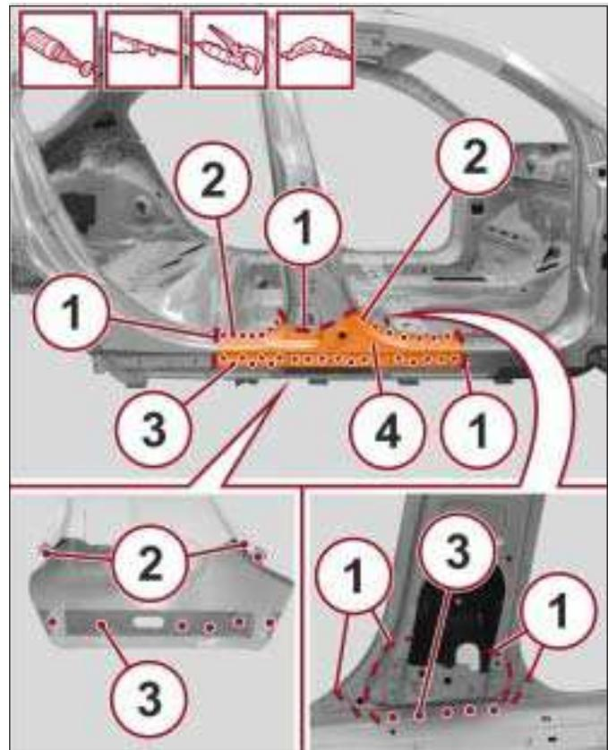
16. With the use of a hammer and dolly block, straighten the edges of the mating components.
