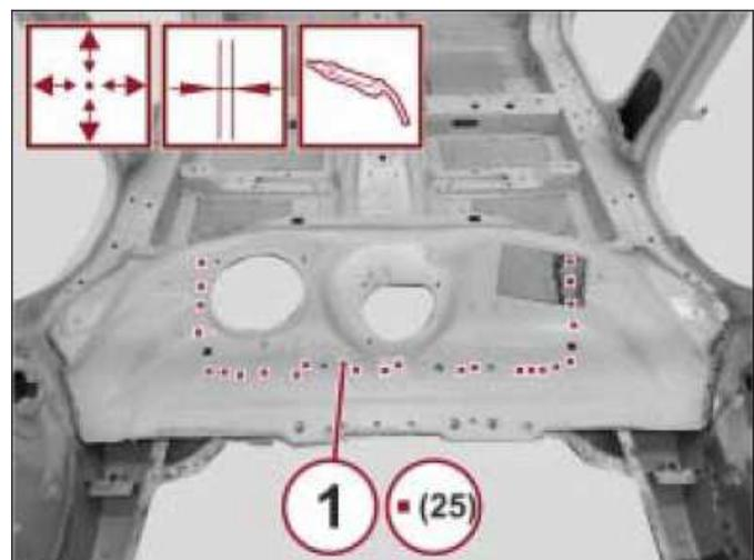
8. With the use of a MIG welder, apply plug welds to the areas (1) shown in the figure.
