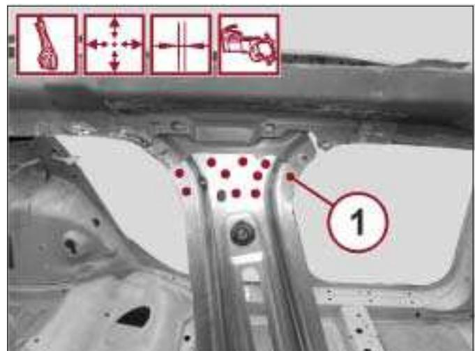
11. Position the inner b-pillar service part correctly on the vehicle and secure it with the self-locking clamps.
