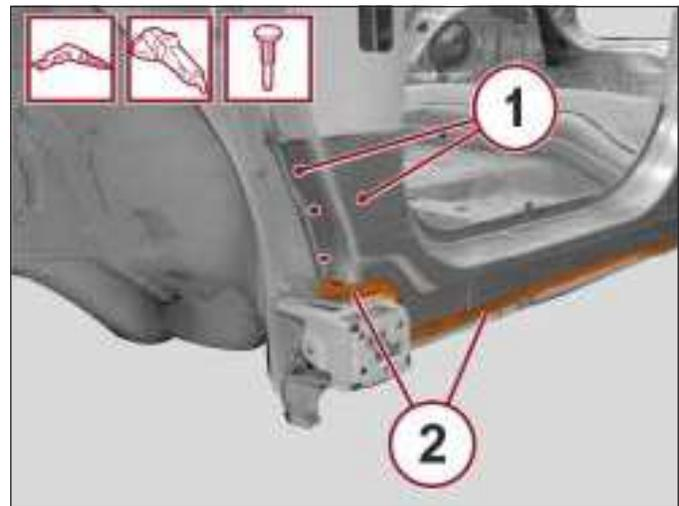
15. With the use of a hammer and dolly block, straighten the edges of the mating components.
