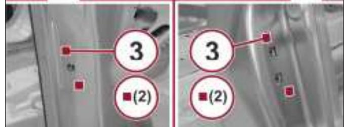
41. With the use of a spot welder, apply spot welds to the areas (1) shown in the figure.
