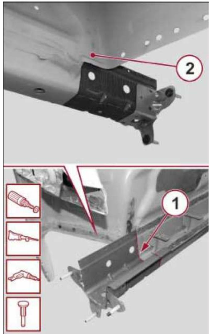
11. With the use of a hammer and dolly block, straighten the edges of the mating components.
