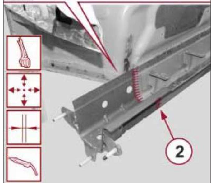
8. Correct any distortions to the sheet metal using a hammer and dolly block.
