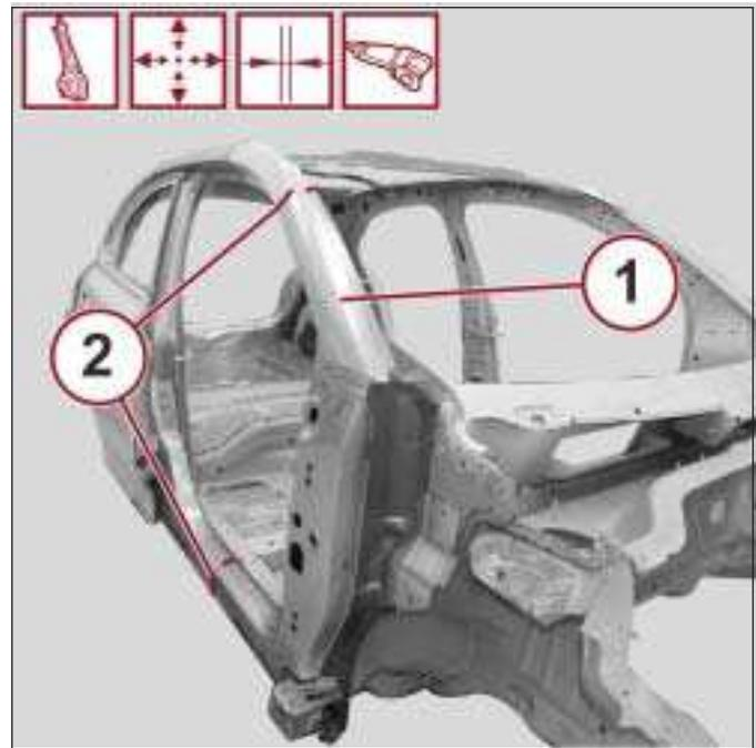
23. Position the external service part (1) correctly on the vehicle and secure it with the self-locking clamps.
