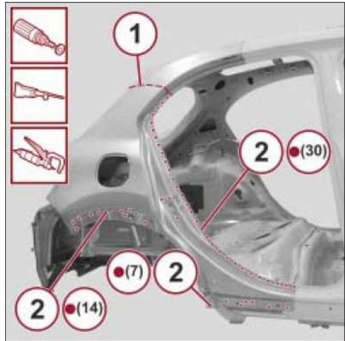
6. With the use of a drill, release the spot welds (1) shown in the figure.
