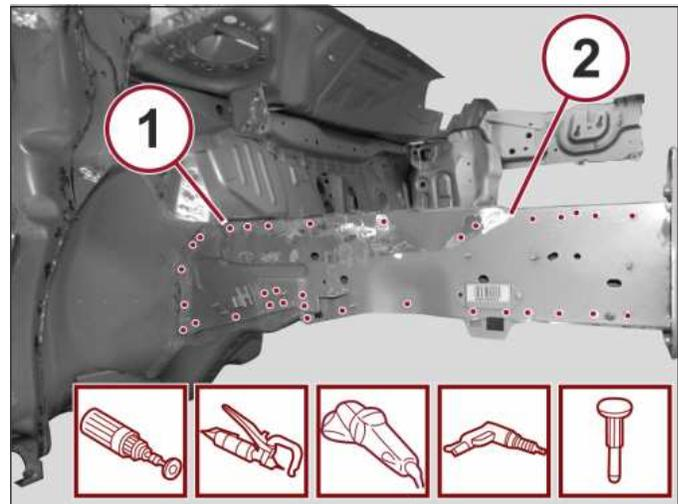
10. Use a rotary brush to remove the paint and gain access to the spot welds.
