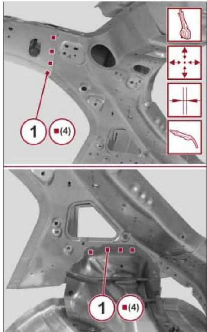
7. Position the service part correctly on the vehicle and secure it with the self-locking clamps.
