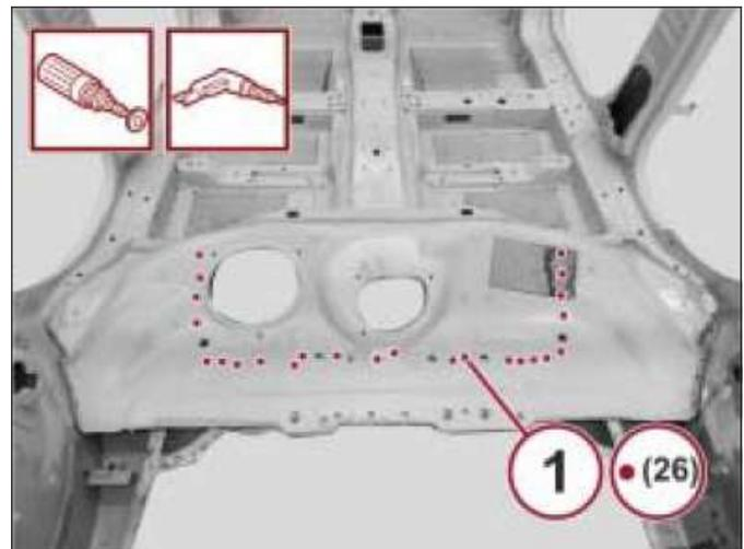
8. With the use of a drill, remove the spot welds (1) shown in the figure.
