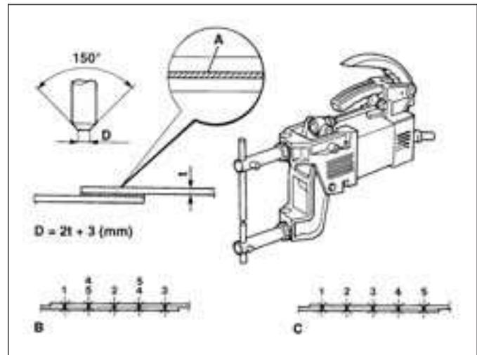
Spot welder, geometric specifications of the electrode depending on the thickness of the panel and the welding sequence.
