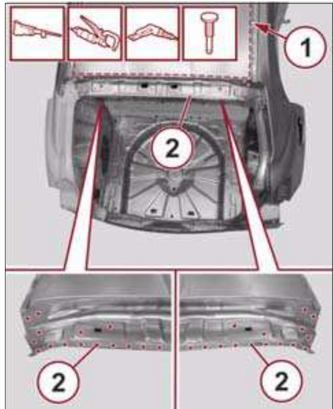
15. With the use of a hammer and dolly block, straighten the edges of the mating components.
