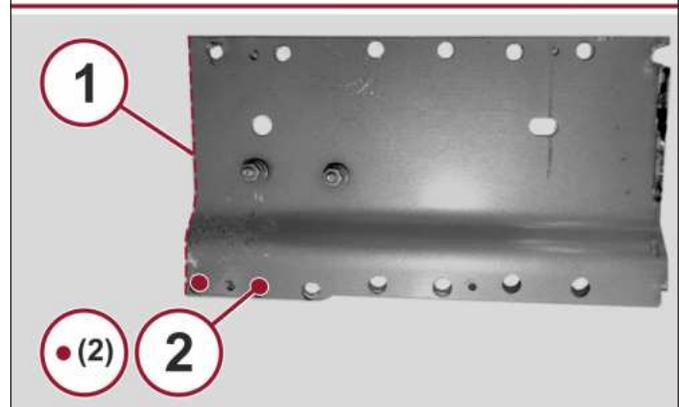
3. Remove the anti-corrosion treatment from the entire perimeter (1) of the inside and outside of the service part using a rotary brush.
