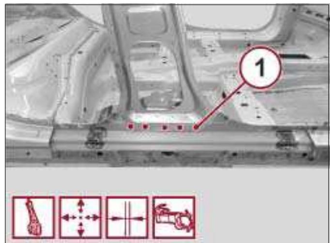
14. Correct any distortions to the sheet metal using a hammer and dolly block.
