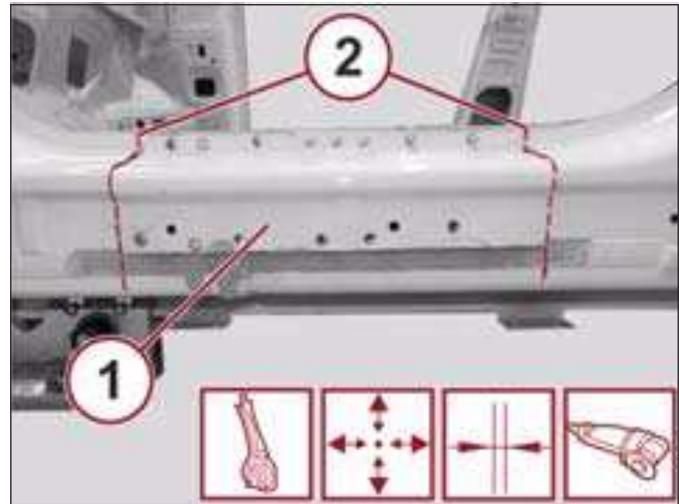
11. Position the body side aperture sill service part correctly on the vehicle and secure it with the self-locking clamps.
