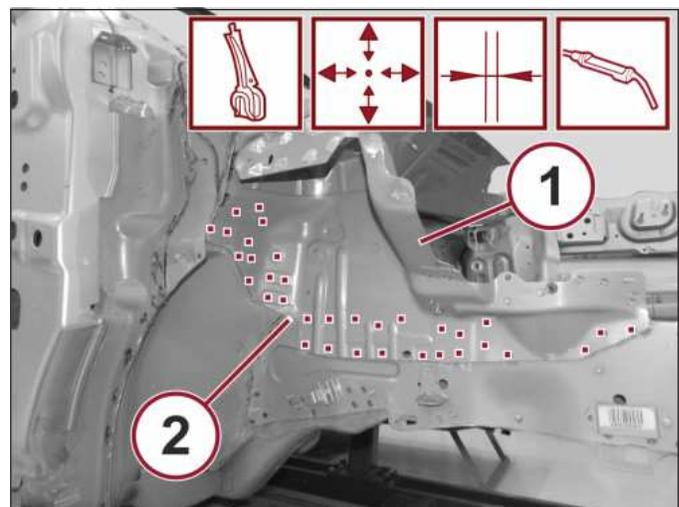
11. Position the service parts correctly on the vehicle and secure it with the self-locking clamps.
