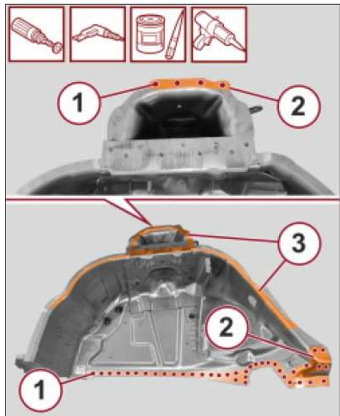
5. Position the service part correctly on the vehicle and secure it with the self-locking clamps.
