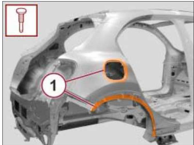
12. With the use of a hammer and dolly block, straighten the edges of the mating components.
