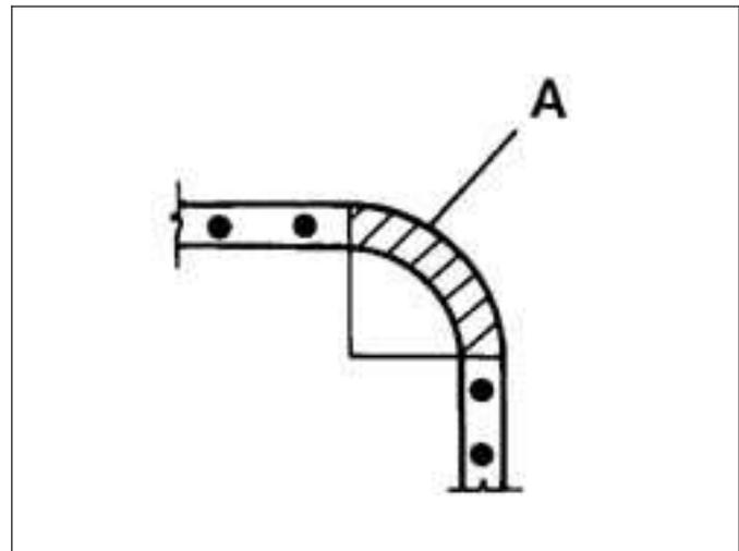
Example of correct spot welding at corners.
