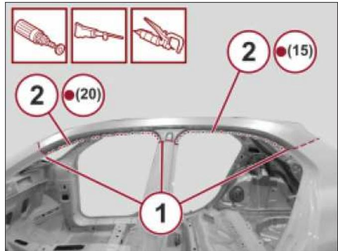
7. With the use of a rotary brush, remove the paint and gain access to the spot welds.
