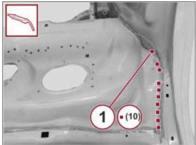
10. With the use of a MIG welder, apply plug welds to the areas (1) shown in the figure.
