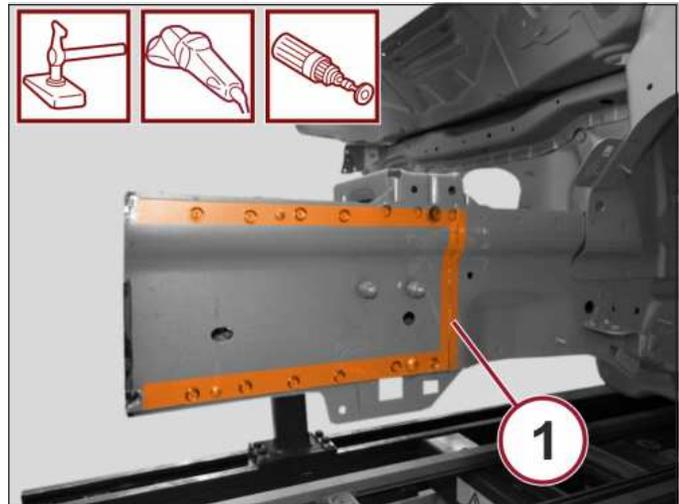
18. Apply corrosion protection to the areas involved in the welding.
