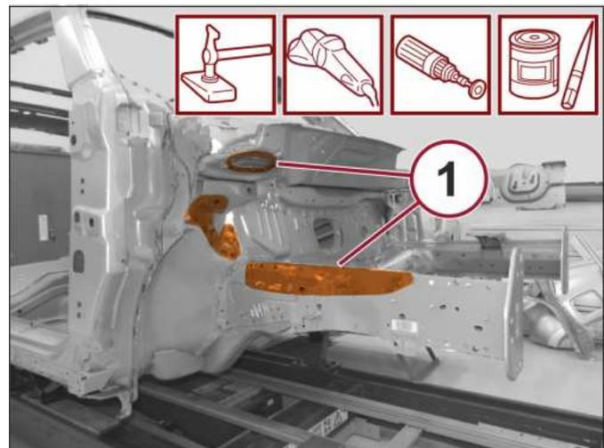
19. With the use of a hammer and dolly block, straighten the edges of the mating components.
