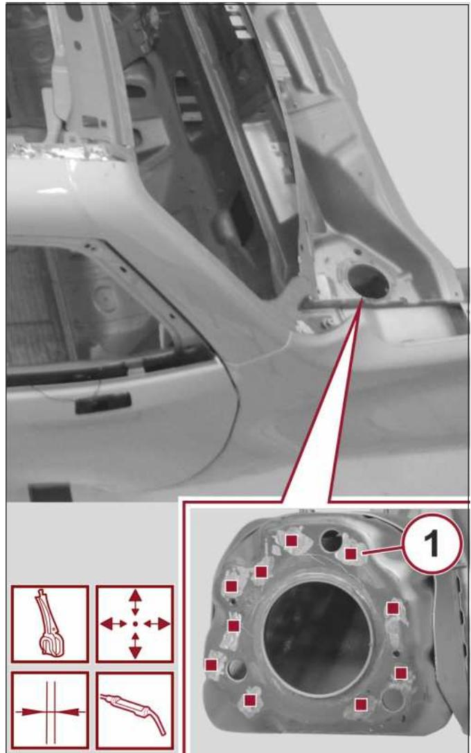
14. Position the service parts correctly on the vehicle and secure it with the self-locking clamps.
