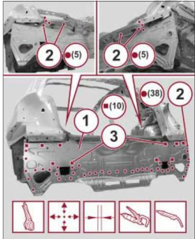
8. Correct any distortions of the sheet metal using a hammer and dolly block.
