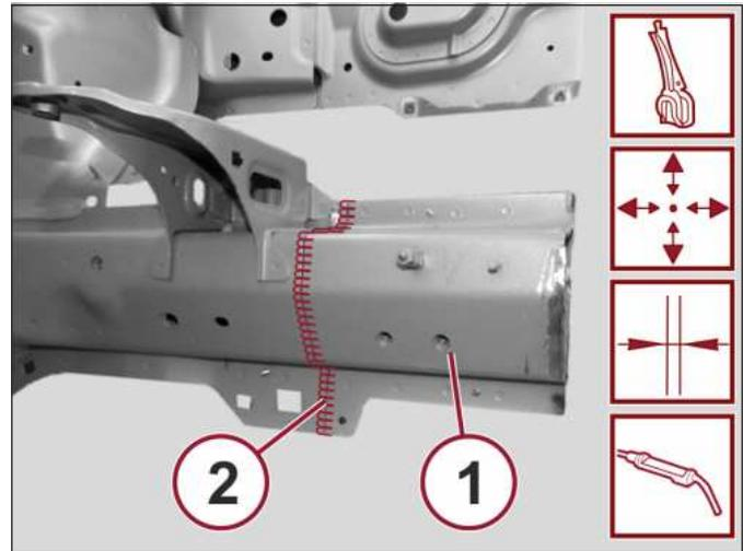
9. Use a spot welder to perform the spot welds (1) where indicated.
