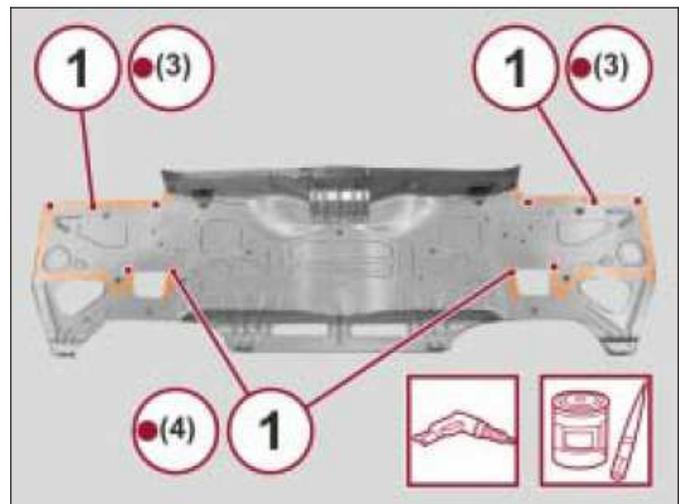
4. Position the inner service part (1) correctly on the vehicle and secure it with the self-locking clamps.
