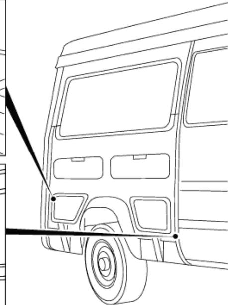
Perform the following step only if side wall paneling is welded with plug welds (SG
