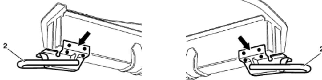
7. Weld towing hook (2) to front longitudinal frame member (arrows).
