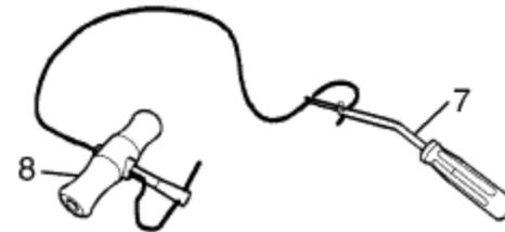
5.1 Support countersupport (7) at top and on sides approx. 30 cm above passage of cutting wire for bead of glue, pull on T-handle (8) on outside in direction of countersupport (7) and cut through bead of glue.
