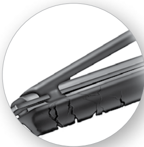
CRACKED RUBBER SPLITS AND/OR SLASHES IN THE RUBBER
