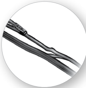
BENT AND/OR CRACKED ARM AND/OR BLADE
