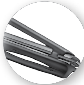
TORN RUBBER PULLED AWAY FROM BLADE (MAKES A SLAPPING NOISE)
